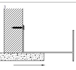
Using a drywall screw (not supplied), mount the housing to the secured structure or blocking at the top of the fixture.
