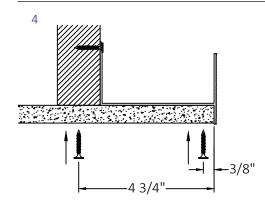
Using a #8 x 1" drywall screw (not supplied), secure the drywall to the secured structure or blocking.
