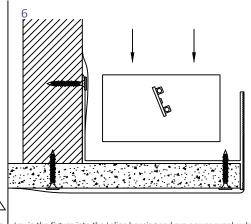
Lay in the fixture into the Lalina housing and run power supply whip to power.
