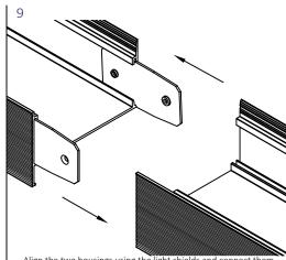
Align the two housings using the light shields and connect then together. Repeat this for all other housings in the run.
