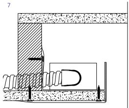
Install the rest of the surrounding sheet rock around the fixture and power on the fixture to make sure everything works properly.
