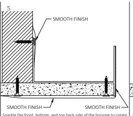
Spackle the front, bottom, and top back side of the housing to create a smooth finish.
